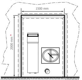
\* Overall height of the alcove is measured from the concrete base
